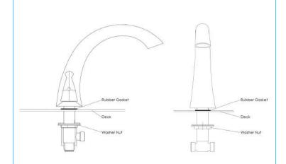
**2.** Unscrew the washer nut and place the rubber gasket and spout above the deck. After, secure the washer nut from underneath the deck.
