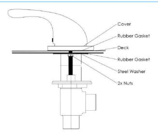
**1.** Unscrew the 2 nuts securing the steel washer and rubber gasket. In this order, remove the steel washer and rubber gasket, place your lever on the deck, replace the rubber gasket and the steel washer. Firmly secure the 2 nuts to hold the fixture in place.
