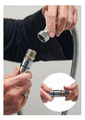
**4)** Connect the hose to your designated water supply (extension hose), and screw it to the opposite side of the barrel.
